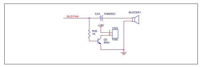
Figure 2-8 Buzzer and Fan Control
